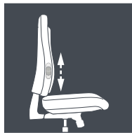
Backrest with integrated height adjustable lumbar support
